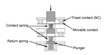
Both NC contacts incorporate a positive opening function. When metal deposition occurs, the contacts are separated from each other by pushing in the plunger.
