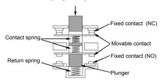
Only the NC contacts have a positive opening function. When metal deposition occurs, the contacts are separated from each other by pushing in the plunger.
